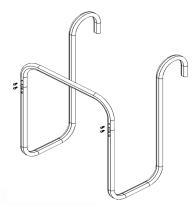
**3)** Gently place your assembled LakeEze<sup>®</sup> Ramp Rack onto your handrail. Ensure the assembly rests against a structural component of the handrail near the bottom of the Ramp Rack.
